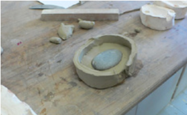
5. Make sure all edges are well sealed with no gaps for plaster to escape through.
