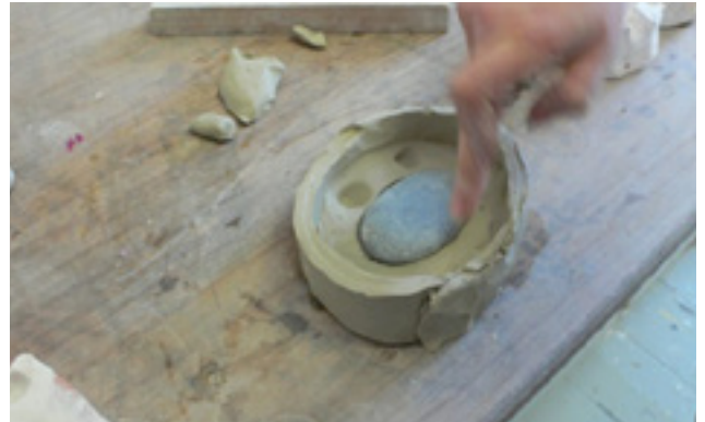
6. Make three small dome-shaped impressions with a finger or small object for mould matching. Pour the plaster onto the mould with the object in it.
