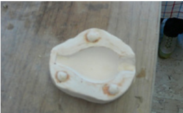
7. This is what the plaster mould would look like with a pouring spout also pressed out. The inverse mould can now be made.
